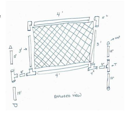
Use the two L shaped connectors at the top left and top right of frame to connect the 4' sections of PVC to the 3' sections.
